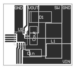
Figure 3. Example CM9330 PC Layout and Component Placement for Standard Application
