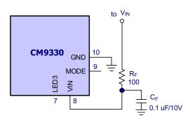
Figure 2. Input Filter Solution
